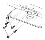
3. Fasten two screws (M4 X L12) at position ①, and then fasten two screws (M4 X L12) at position ②.
